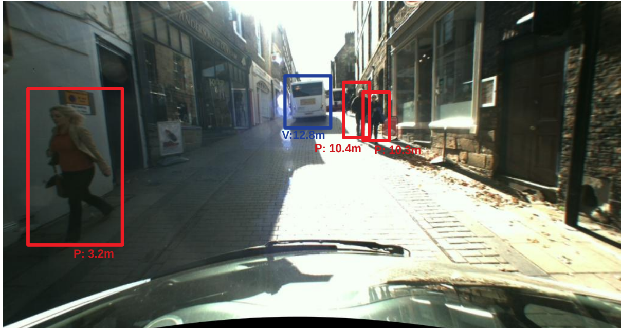
Figure 2: Illustrative polygon outline of the detected scene objects, with distance displayed and abbreviated class label inset, drawn on the left (colour) image. all the files as a “batch” without requiring a user key press or similar.
