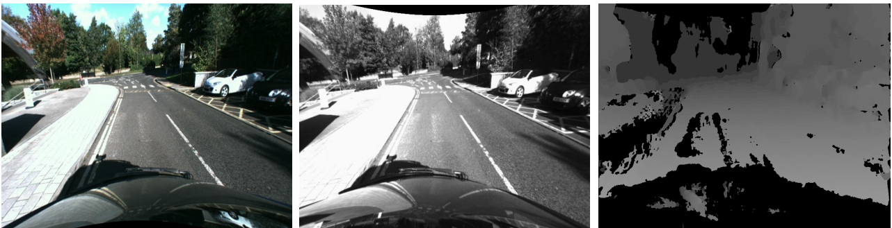
Figure 1: Example left (colour), right (greyscale, rectified) and corresponding disparity calculated using the example python code provided for the assignment.
