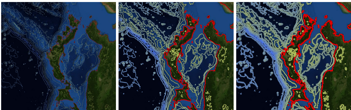
Figure 4: Earth surface elevation represented using isolines wrapped into tubes with varying radii: left: 4707, middle: 14588, right: 26054.
